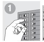
Before beginning TURN OFF POWER to the light from fuse or circuit breaker
