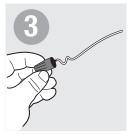
Remove fixture from outlet box. Attach wire nuts to end of each conductor wire.
