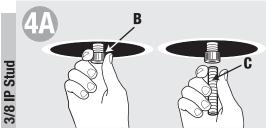
3/8 IP stud: Screw reducer (B) onto stud. Tighten by hand. Screw nipple (C) into reducer.
